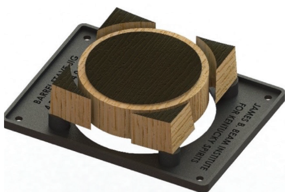
Figure 1. CAD rendering (left) and fabricated (right) stave disks secured to a 3D-printed jig for machining on a computer numeric control router table.
